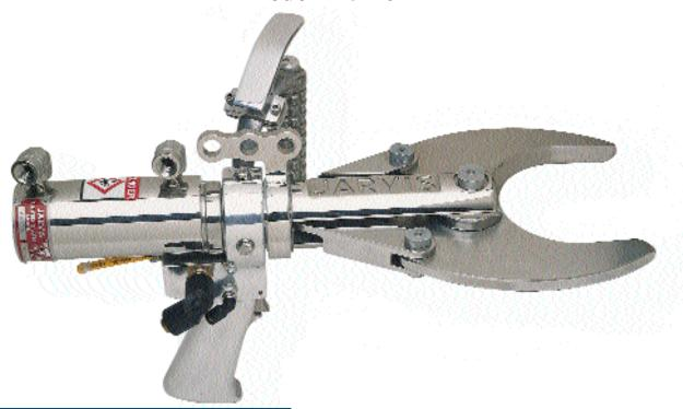
The Jarvis Model 425-16 - hydraulic powered hock cutter for sheep.
