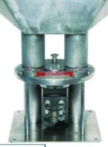
The Jarvis Model HCC-1 electric-hydraulic powered chitterlings cutter
