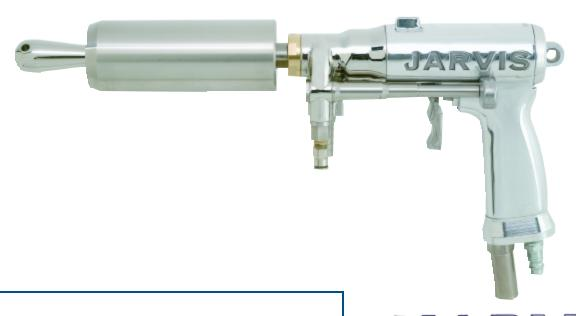
The New Jarvis Model HBD-1 - for the cutting out of hog bungs.
